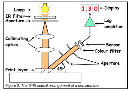
Light reflected by the printed surface is collected at an angle of 45° to the surface, as defined by a pair of apertures. The spectral character of the 45° light is analysed using optical filters to determine the amounts of light in four bands of wavelengths; red, green, blue and visual. National and International Standards establish the characteristics of the filters and of the weighting functions.
